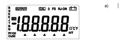
UTPUT: The display of this symbol denotes that the Simulator is in an output state.
