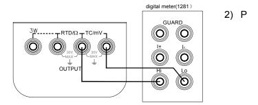
ress the keys (**FUN**) { (**RANG**) first, and then press t he key (**POWER**) to enter the simulator in a state of 1V output calibration when the symbols OUTPUT, CAL 0', 'ON' and the unit 'V' appear in the display.
